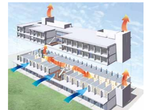
Eco-shaft A natural ventilation system using the updraft of air heated by solar energy.
